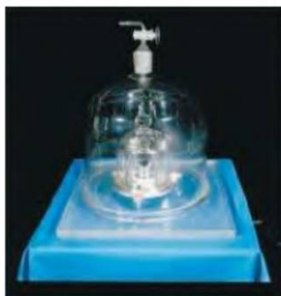
By international agreement, this metal cylinder, stored in Paris, is the definition of the kilogram.
